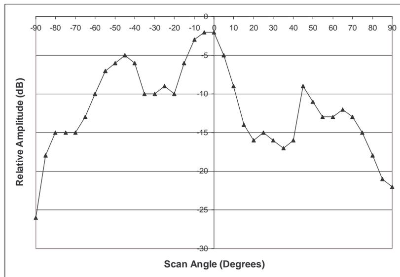
Figure 2 Radiation Pattern for 65.5 GHz 4 Element Patch Array
