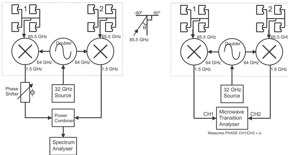
(a) IF Beamsteered Receiver/ Monostatic Direction Finding System
