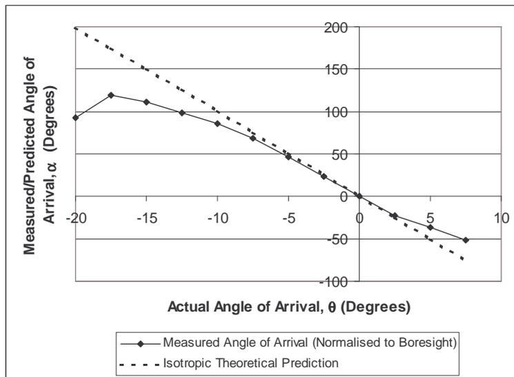
Figure 5 Phase Results Between Antennas 1 and 2 Measured at 1.5 GHz IF
